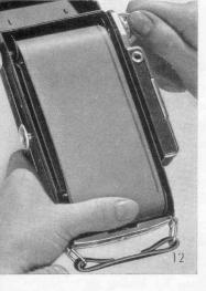
take-up spool. Tighten the protective paper by turning the film winding key (1) several times. Close the camera back. When opening the slide (26) in the camera back you will see two film windows, which serve for verifying the number of pictures made. Turn the winding key until number "1" appears in the first film window (24).
